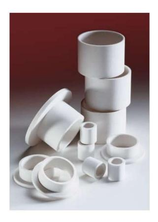
Rulon® 1439 is a white FDA compliant material that is suitable for immersed service with better wear characteristics than most other PTFE compounds. Its color makes it aesthetically pleasing for food and pharmaceutical applications.
